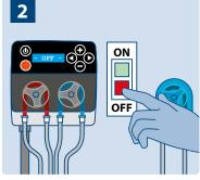
Switch **OFF** external dosing equipment. For integral pump disconnect detergent and rinse aid.
