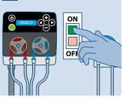
Switch **ON** external dosing equipment. For integral pump reconnect detergent and rinse aid.
